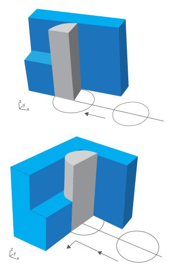
At this intersection, large engagement would cause tool chatter and even breakage. Using CAD CAM software to generate the corner avoids an abrupt stop and change of direction. It also keeps a constant arc of engagement while providing smooth chatter free cutting and long tool life.
